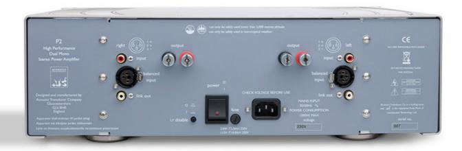
The output stage on this ATC, like its range mates on the back of the company's active loudspeakers, is based around three pairs of MOSFET transistors in a dual mono arrangement so as to minimise interference between channels. It has a larger power supply than the P1 and higher voltage capacitors but is based on the same circuit and component types. Both amps are wide bandwidth, class AB designs of the not to be messed with variety.
